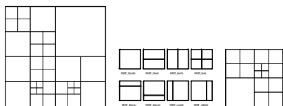
Fig. 3 Standardized MPEG-H HEVC / ITU H.265 video codec: Block-based hybrid transform-entropy video encoder with motion-compensated prediction; Operational ORD points for 12 different quantization parameters QP and bitrates R in encoding/decoding test sequence Vidyo1 ; Adaptive frame partition into Coding Blocks (CB), PredictionBlocks (PB), TransformBlocks (TB) [8].
